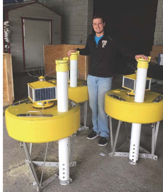
Figure 2. CREST-CACHe Research Buoys are deployed in freshwater and near-shore marine aquatic ecosystems. Buoys are arrayed with high-tech sensors to collect general water quality data at high sampling frequency.
