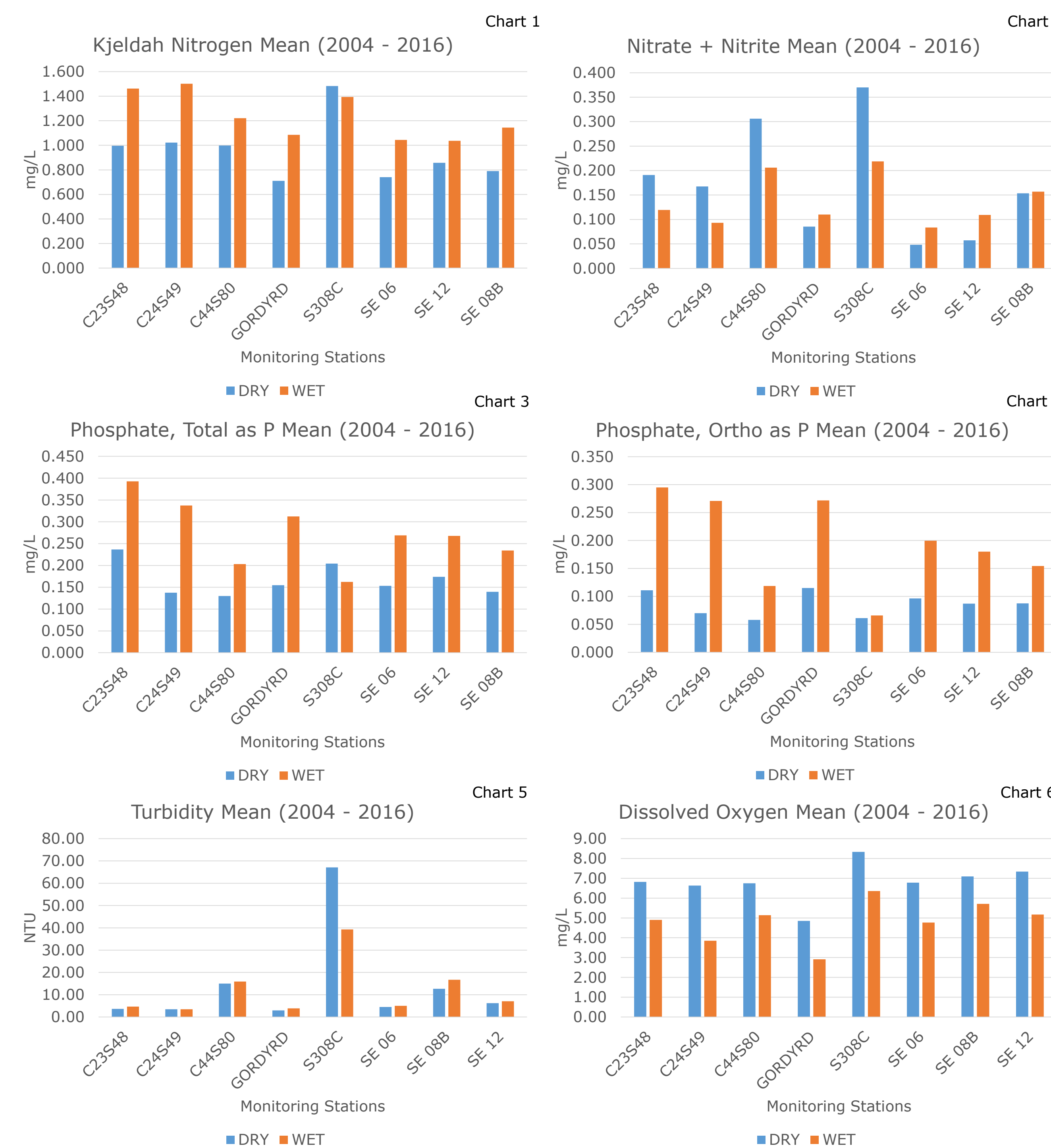
Charts 1 – 6. Average concentrations of nutrients, turbidity, and dissolved oxygen for the wet (Jun – Nov) and dry (Dec – May) seasons of 8 monitoring stations on the St Lucie Estuary watershed from 2004 - 2016.
